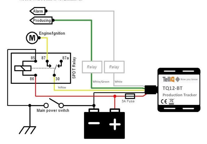
NOTE! The unit consumes < 4mA when the machine is not in use
