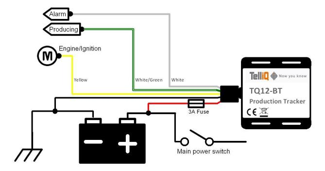
NOTE! The unit consumes < 6mA when the machine is not in use
