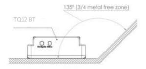
Best TQ12-BT mounting position is outside of vehicle without any metal above the device. Recommended deviation from horizontal axis of vehicle is max 3-5°, as shown in Figure.
